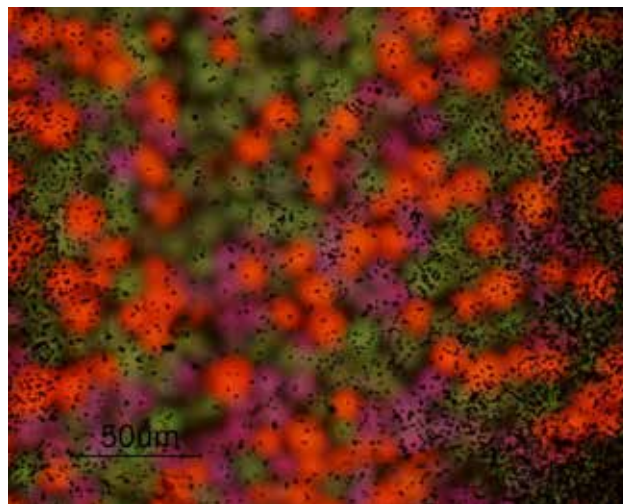
Microscopic study of the silver grain side of a Cinécolor (Autochrome) 35mm sample, ca. 1932 (HTW - University of Applied Sciences, 2016)
