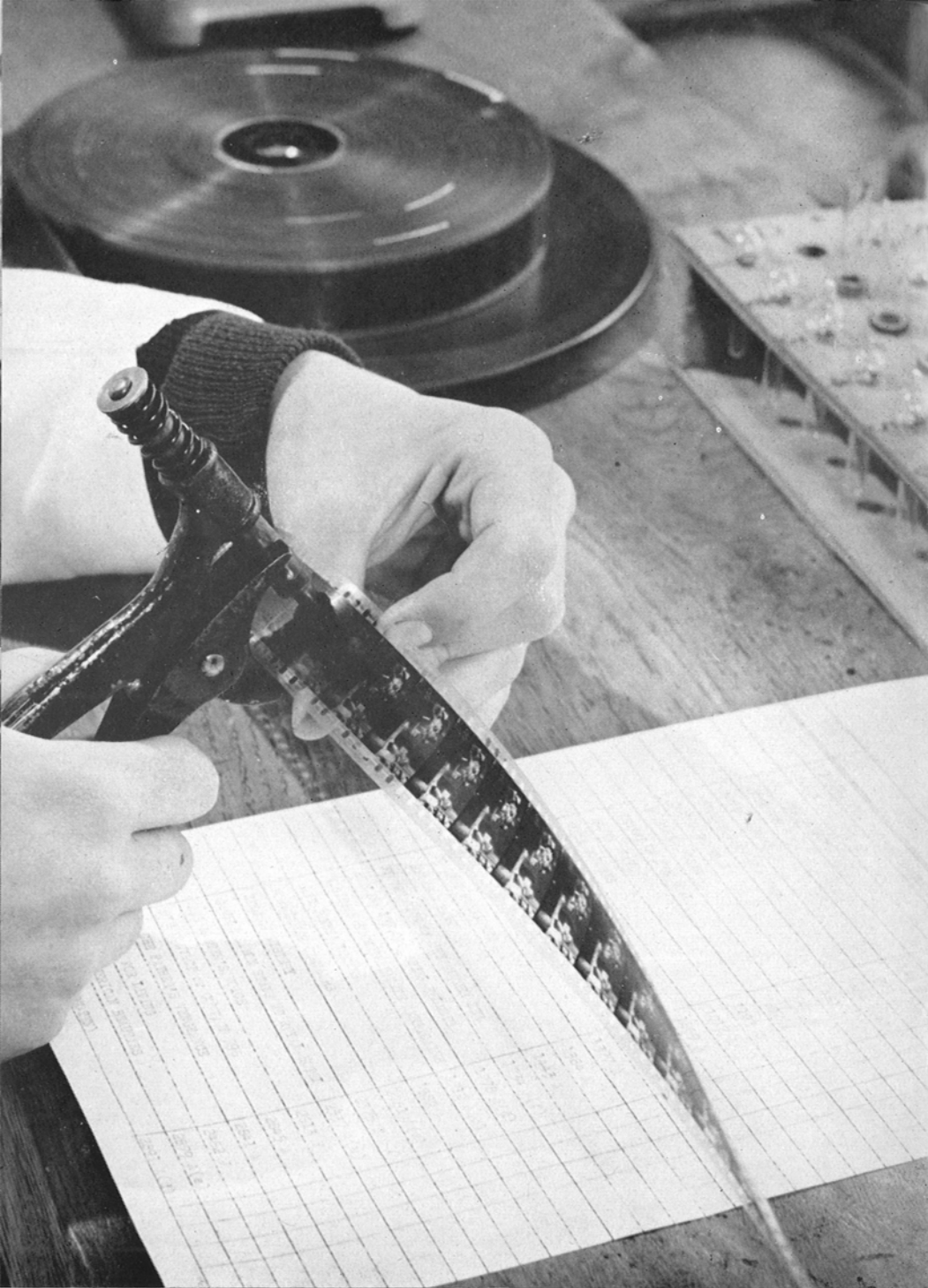
4. Film Stability test for nitrate film: taking sample punching
