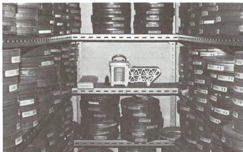
The thermo-hygrometer records temperature and humidity in a nitrate vault. Notice that films are stored flat and not on end, to avoid distortion caused by pressure from the weight of the film.
