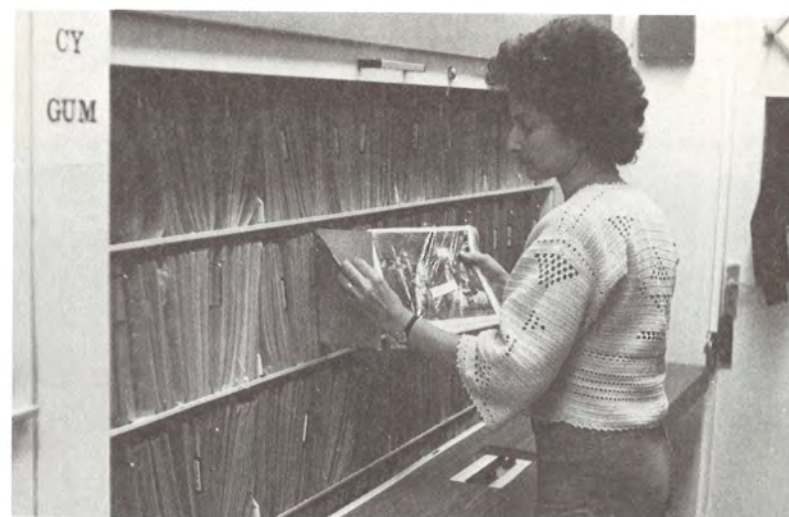
Space is usually a problem for the growing quantities of documentation materials. One solution is compact automated shelving. The Sperry Remington Lektriever storage system, used here for stills, returns the needed shelf at the touch of a button. It requires a reinforced floor to carry the heavy weight.
