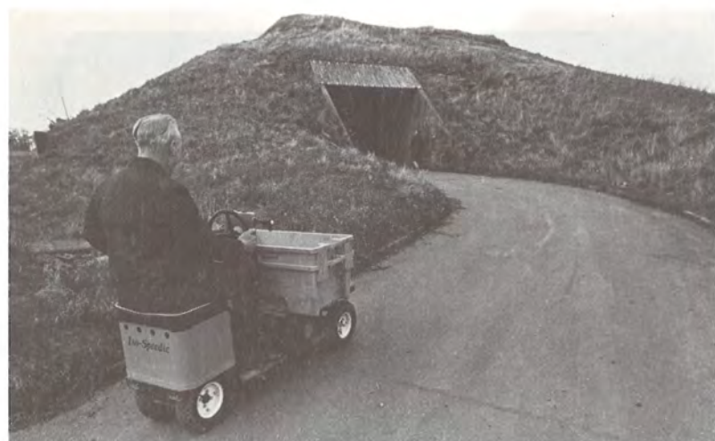
An electric trolley used to transport films from a van parked on the road to the vaults. Vaults should be located as far as is practical from major industrial areas to avoid the chemical dangers of pollution. Nitrate vaults must be at a distance from congested areas to avoid risks to the population from fire and the noxious fumes that accompany it.
