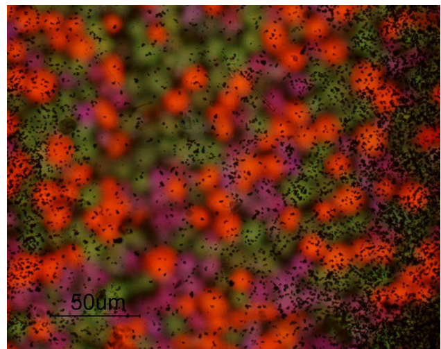
Microscopic image of Cinécolor (which is essentially Autochrome)
