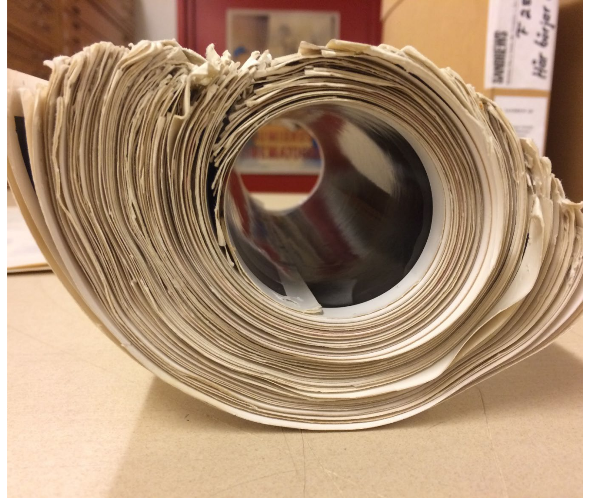
Extreme case of poor storage and dry climate
